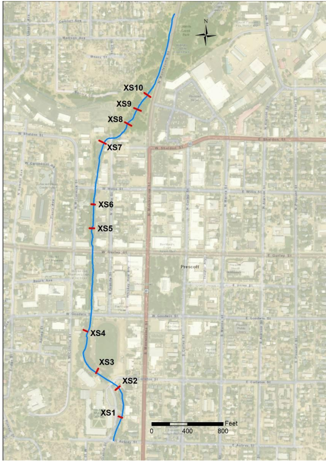
Figure 4. Location of channel cross sections.
